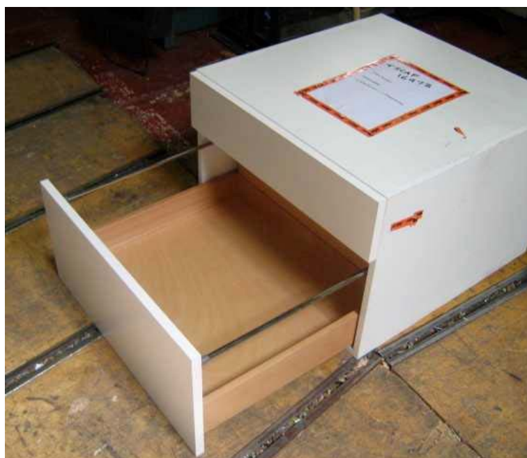
Plate 1: 551H5101B TANDEM Runner Hook + Peg Variant With Integrated BLUMOTION For Wooden Drawer (Front View)
